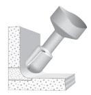
The processed piece is then cut leaving 2–3mm of edge, which is glued on the countertop, where we have previously made a groove 2–3mm deep and 25mm wide.
