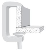
In case of Kerrock sheets which contain metal particles (Metal, Luminaco S and Marble effect), the appearance of the surface and edge of the sheet differ, so make sure the edge is not visible when making joints. There are two ways for doing that:
